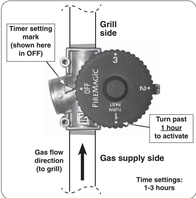
Fig. 1-2 Vertical setup
